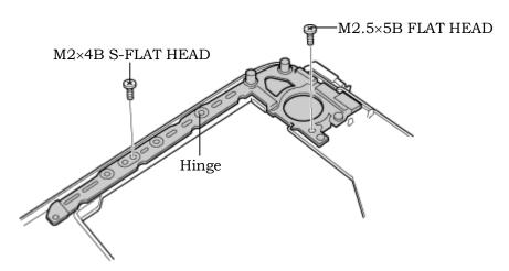
Figure 4-49 Removing the hinge
